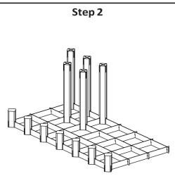
Line up and insert the wood rack pieces into the metal frame. Use a rubber mallet to install into the metal cross frame. Repeat until all wood rack pieces are installed.
