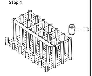
Insert the second section of the metal frame into the first and using a rubber mallet complete the installation into the wood pieces.
