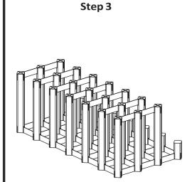
Very important! Insert one section of the metal frame only half way down into the wood pieces.
