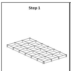
Assemble the bottom metal frame on a flat surface.
